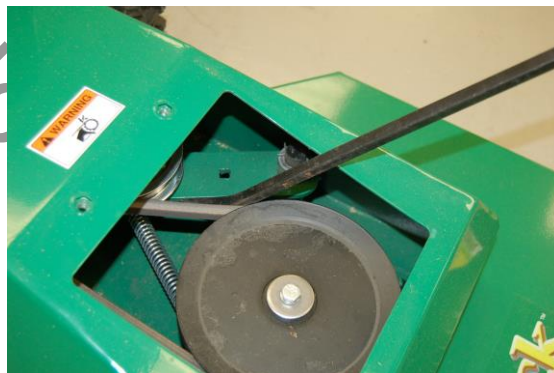
Removing tension on the blade belt
