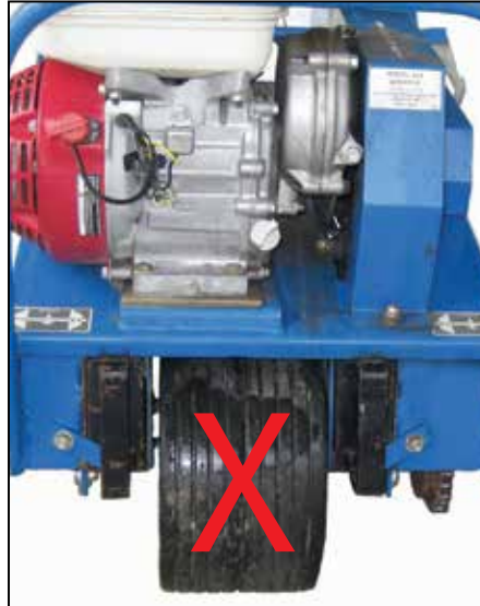
Compare how the outboard drive wheels eliminate both centre wheel slip and abuse from ramp loading with the tines engaged.
