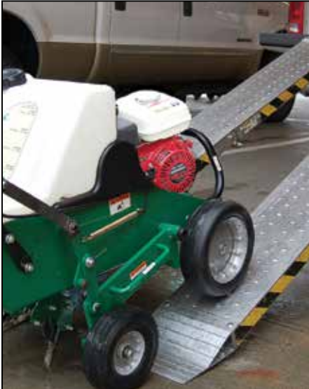
Compare how the outboard drive wheels eliminate both centre wheel slip and abuse from ramp loading with the tines engaged.
